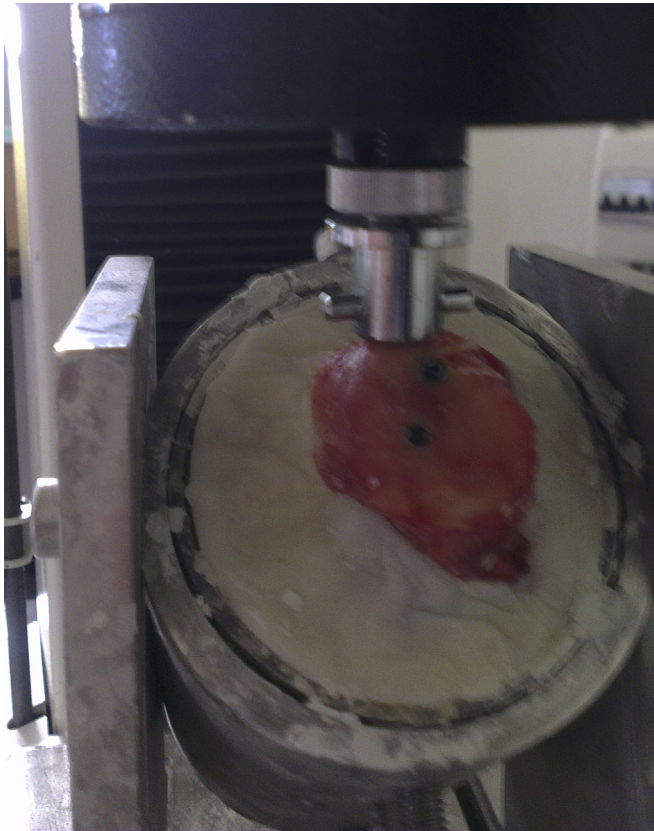
Fig. 1. The experimental setup showing the cup-shaped impactor applying a force to the talar head at 45° to the long axis of the talus.
