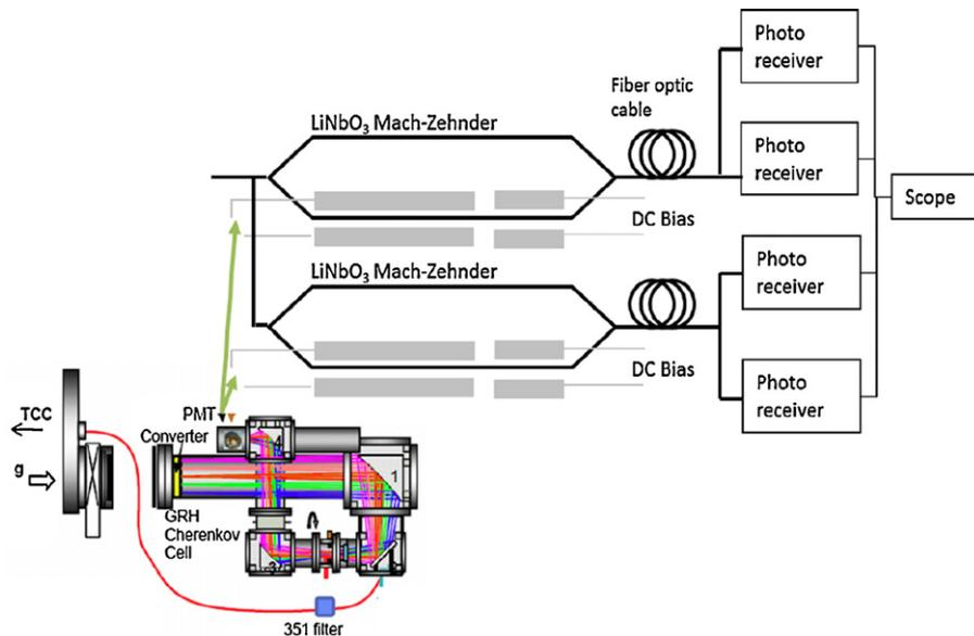
Fig. 2. GRH diagnostic hardware layout.
