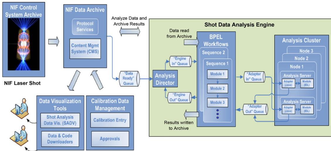
Fig. 1. Shot Data Analysis automated engine workflow.
