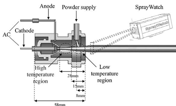
Fig. 1. Schematic of supersonic plasma spraying gun.
