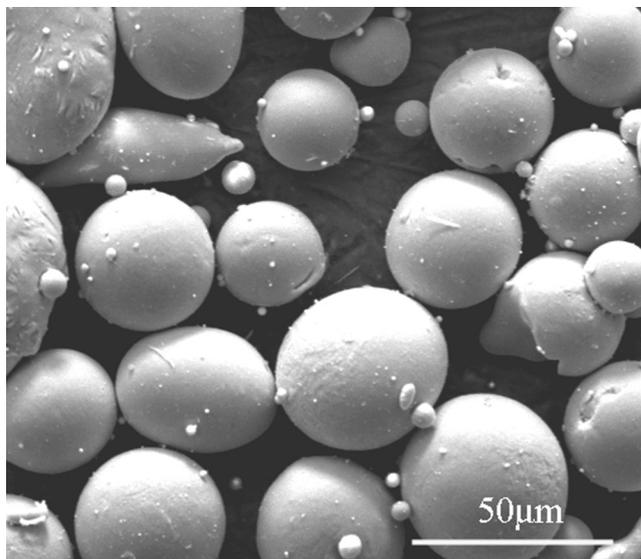
Fig. 3. Morphologies of Fe-based powders.
