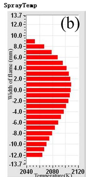
Fig. 2. Monitor of melting particles by SprayWatch: (a) the average values of temperature and velocity of the particle; (b) the proof of the temperature of melting particle temperatures.
