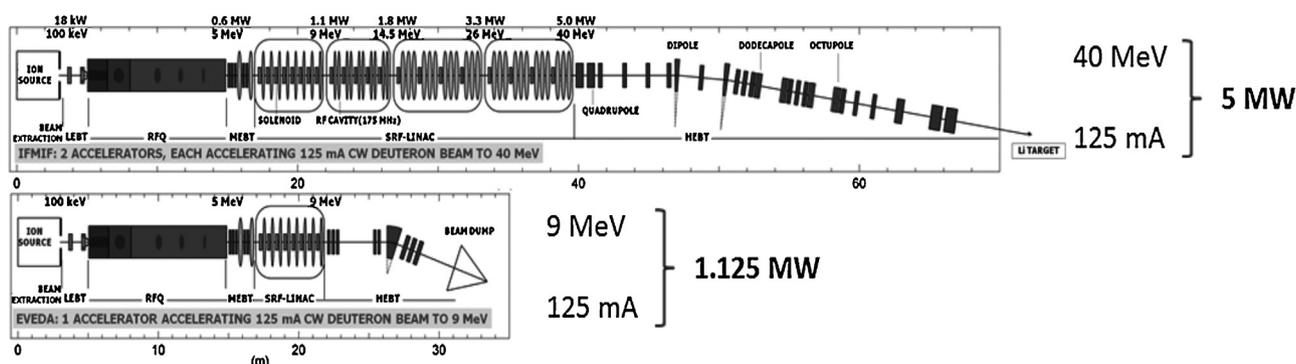
Fig. 1. Features of the 2 accelerator systems designed for the IFMIF plant (top) compared to the Linear IFMIF prototype accelerator (“LIPAc”) being manufactured, installed and commissioned in the IFMIF/EVEDA Project (bottom) [9].
