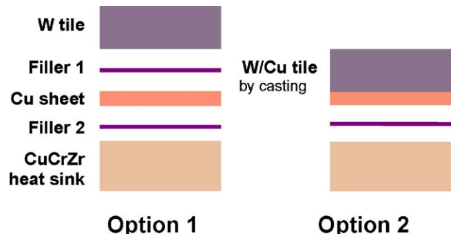
Fig. 3. Two schemes of armoring by brazing.
