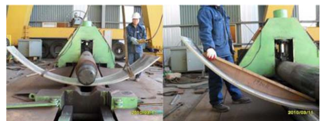
(a) Roll bending of upper/lower shell
