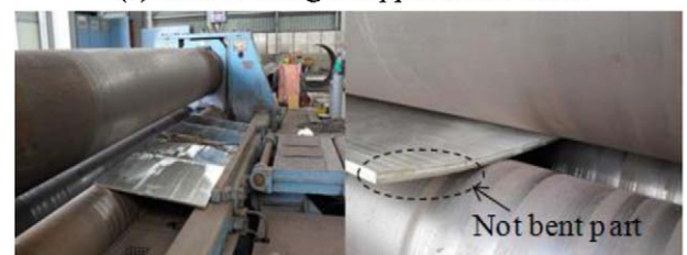
(b) Roll bending of central shell
