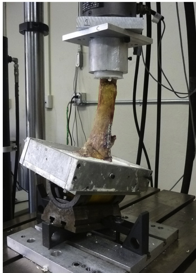
Fig. 2. Prepared specimen (with an implanted locking plate) secured within the testing apparatus.
