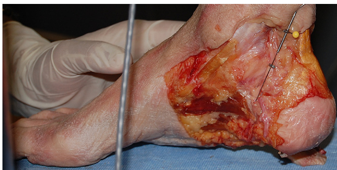
Fig. 1. Posterior tibial nerve with differential variable reluctance transducer. Image of right-footed specimen mounted on the materials testing system (not shown) with the foot in the neutral position and the differential variable reluctance transducer mounted on posterior tibial nerve as described in the “Materials and Methods” section. The output of the differential variable reluctance transducer was recorded in this position to give the initial or reference length, after which the foot was maximally pronated, and the differential variable reluctance transducer output was recorded to calculate the change in the length or elongation of the posterior tibial nerve.
