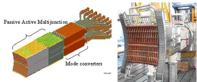
**Fig. 2.** PAM launcher equipped with its side protections on the equatorial lateral side of the front face and with its vacuum flange at the back. The structure is composed of two components bolted together: (1) the Passive Active Multi-junction (PAM) and (2) the Mode Converters.
