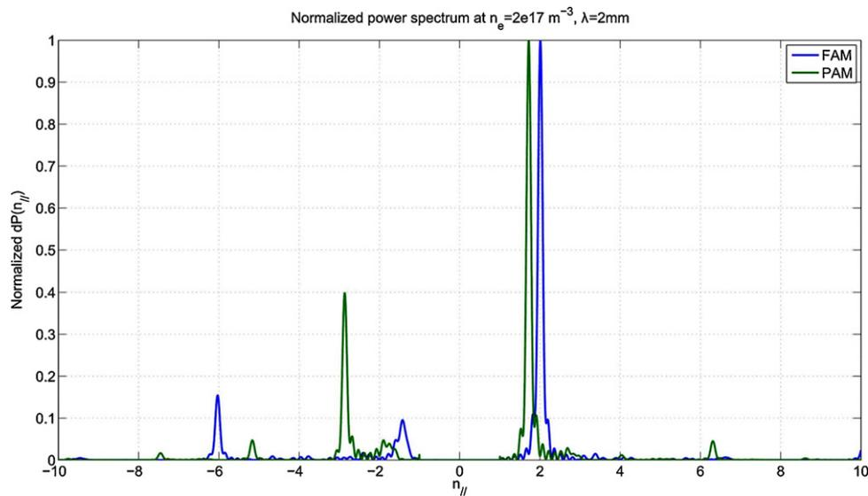
**Fig. 1.** Normalized to unity power spectrum for the Full Active Multijunction (FAM) and the Passive Active Multijunction (PAM). Plasma edge density is modeled with an electron density of  $n_e = 2 \times 10^{17} \text{ m}^{-3}$  ( $n_{\text{ecutoff}} = 1.7 \times 10^{17} \text{ m}^{-3}$ ) and a 2 mm scrape-off e-folding decay length. The normalized power directivities are respectively 0.72 and 0.67.
