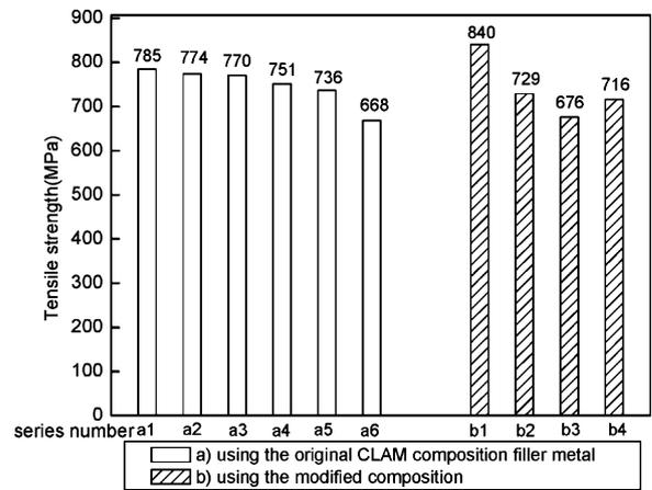
Fig. 2. Ultimate tensile strength of joints under identical conditions.
