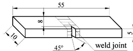
Fig. 3. Shape and dimensions of CIT specimen (a) a5 (b) b3.
