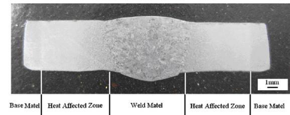
(a) Cross-section of TIG weld joint
