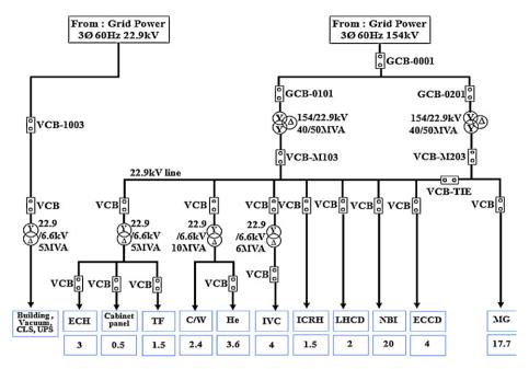
Fig. 1. The power distribution of the KSTAR.
