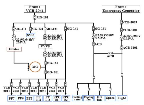
Fig. 2. Power distribution diagram of MG.
