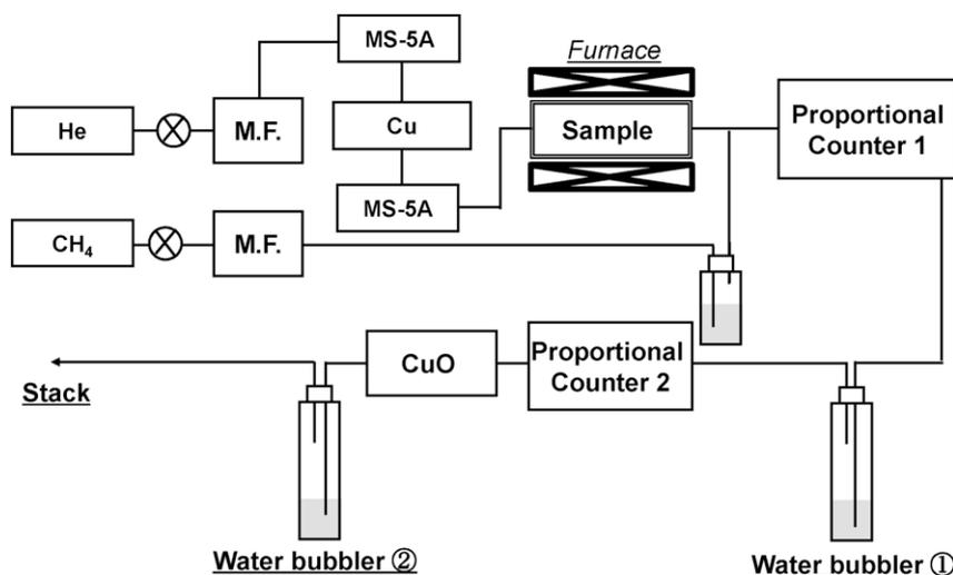
Fig. 1. Schematic drawing of tritium-TDS system.
