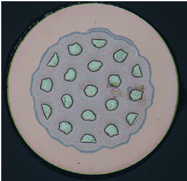
Fig. 2. The cross-sectional area of Nb 3 Sn strand before heat treatment.
