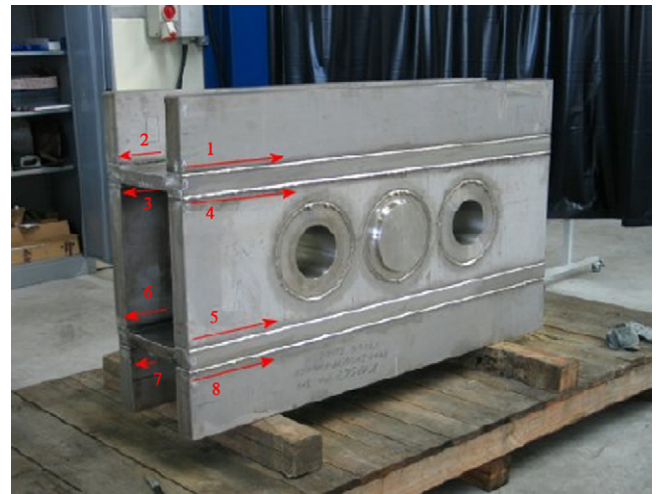
Fig. 3. Tack weld position references.
