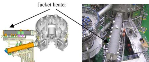
Fig. 3. Jacket heaters system for the pumping duct.
