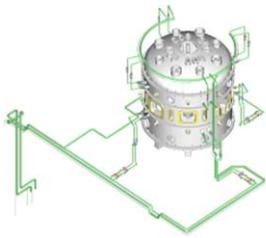
Fig. 2. The piping diagram for the water baking system.
