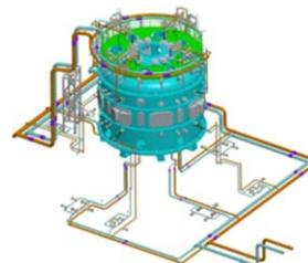
Fig. 4. The piping diagram of the GN<sub>2</sub> line and tiles of the inboard limiter.
