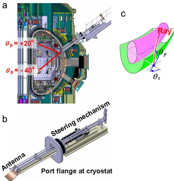
**Fig. 1.** CAD model of the ECRF launcher for JT-60SA. (a) The poloidal cross-section of the JT-60SA tokamak where one of the ECRF launchers is installed. (b) An ECRF launcher consisting of the antenna portion inside the vacuum vessel and the steering mechanism outside the vacuum and support structures. (c) Definition of the toroidal and poloidal injection angles.
