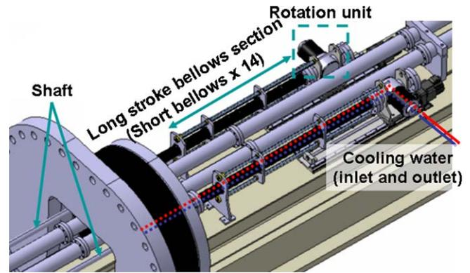
**Fig. 2.** Schematic view of the steering mechanism. A rigid shaft connected to the M1, which includes cooling water lines (inlet and outlet), is contained in the long-stroke bellows section and bended at the rotation unit.
