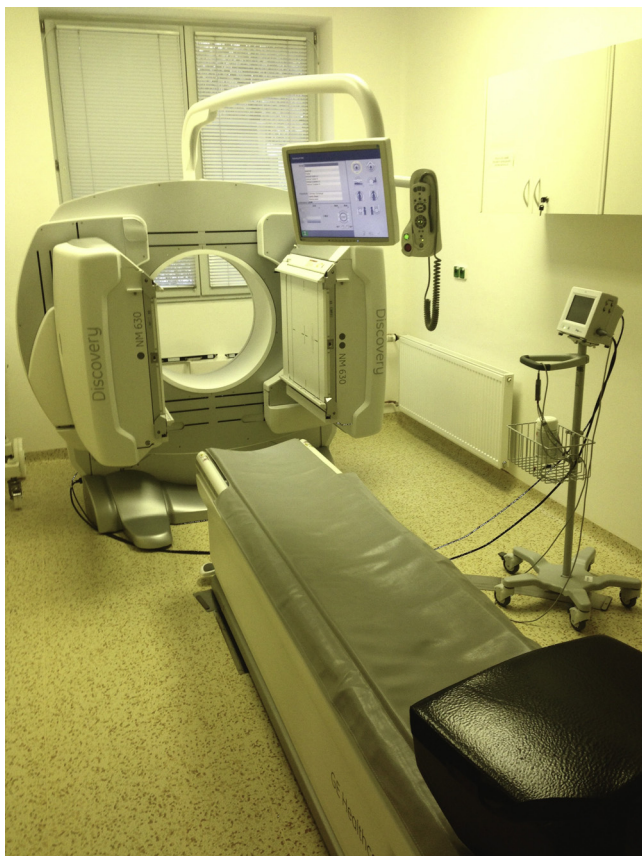
Fig. 1 – Conventional two-detector SPECT camera (Discovery NM 630, GE Healthcare).
