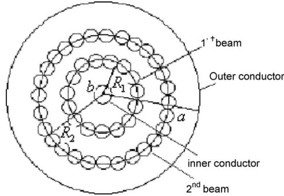
Fig. 1. Schematic cross-section of the CGTB.
