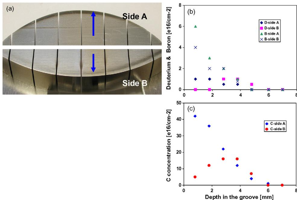
Fig. 2. Deposition belts in gaps of castellation on both sides of Slice 2 (a) and deposition profiles of deuterium and boron (b) and carbon (c). The deposition belts near the top of the gap on Side A and Side B are marked with arrows.
