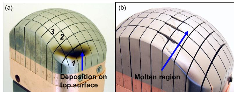
Fig. 1. W macro-brush limiter after the first (a) and second (b) exposure at TEXTOR. Slices analysed with IBA are numbered 1–3.
