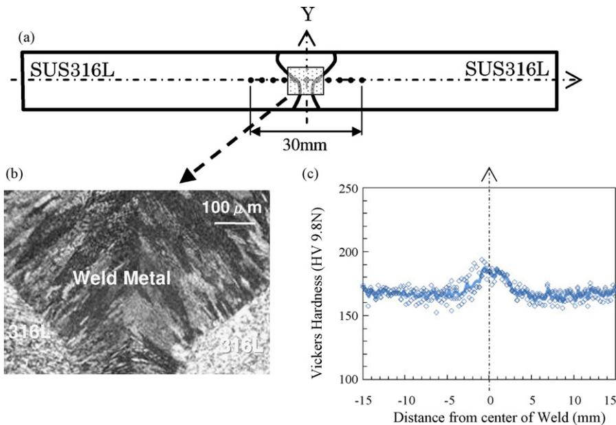
Fig. 2. Hardness distribution and cross-sectional macrostructure of weld joint.
