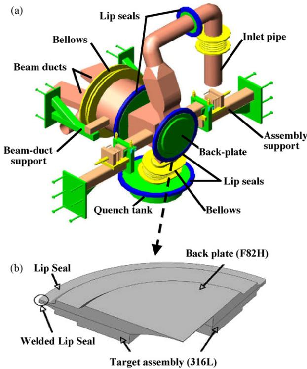
Fig. 1. Overview of Li target assembly (a) and a quarter of the back plate with lip seal (b).
