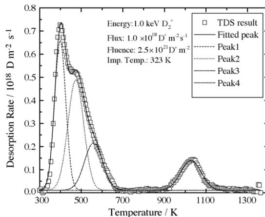
Fig. 2. TDS spectra of D<sub>2</sub> for  $D_2^+$  implanted WC with fitted peaks.
