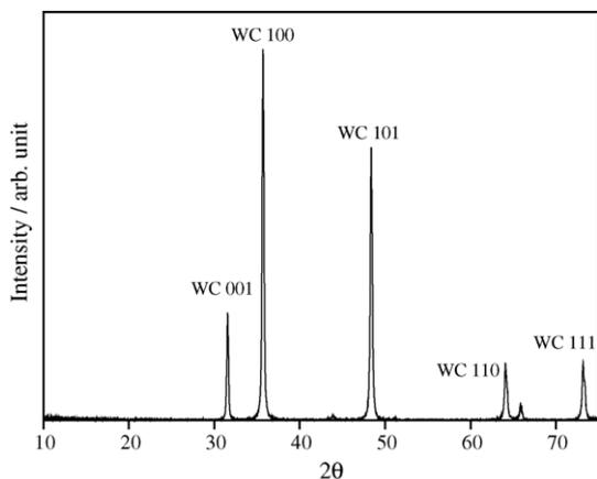
Fig. 1. XRD pattern of WC after heating treatment at 1373 K.
