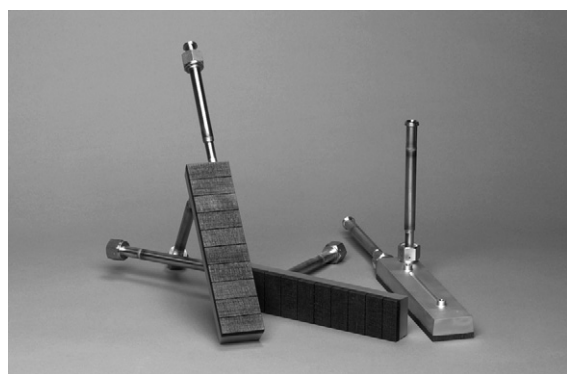
Fig. 1. Photograph of target elements type 4S with the cooling water inlet in axial direction and the perpendicular arranged outlet tube. The right hand element shows the 10 flat CFC NB 31 tiles.
