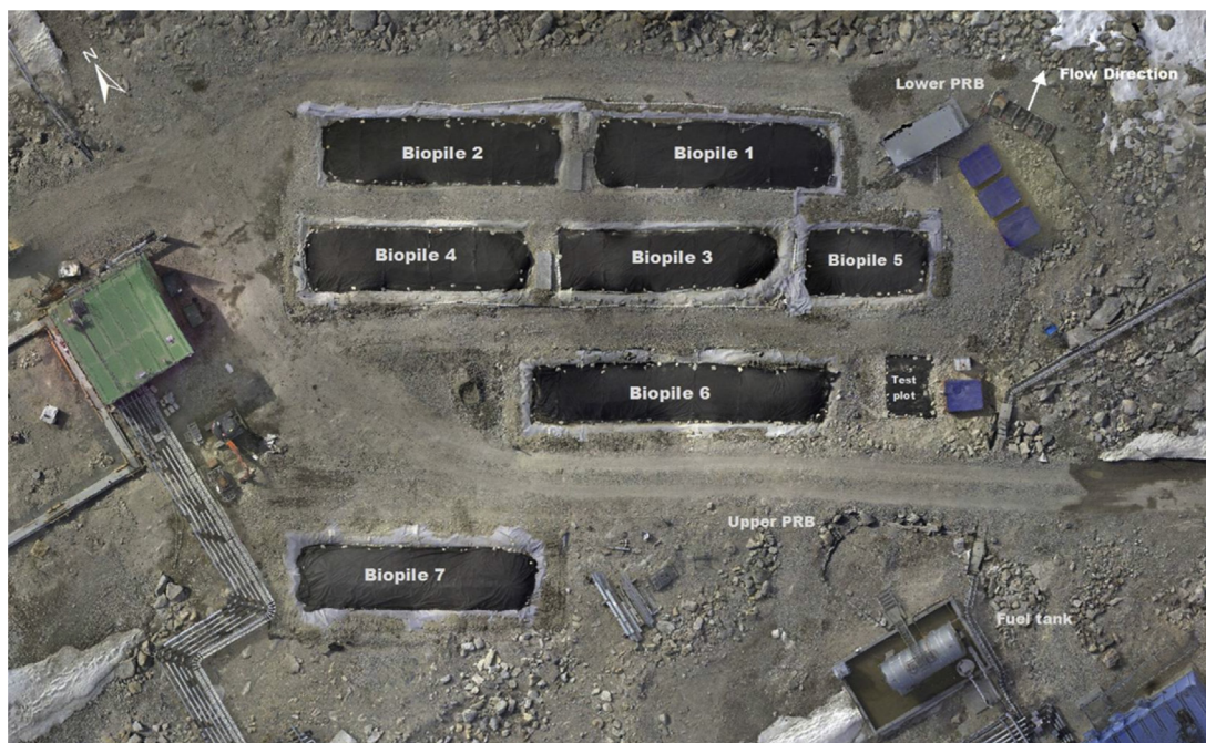
Fig. 1. Remediation site showing: fuel tank (source of the 1999 fuel spill), contaminant flow direction, upper and lower PRBs, seven biopiles and test plot. Black upper covers shown are GTX2 or GTX4 (see Table 1).
