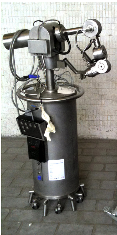
Figure 1 Prototype of the manual surgical robotics developed by the orthopaedic surgical team.
