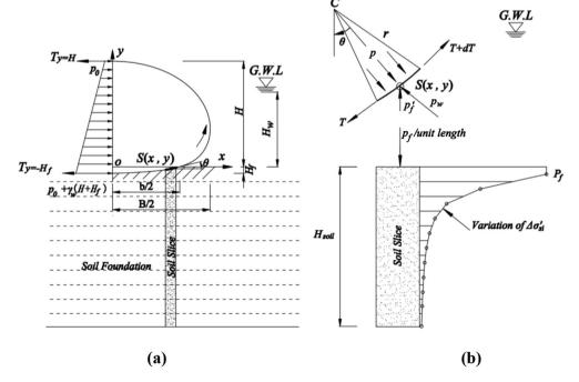
Fig. 1. Free body diagram (a) for half of a geotextile tube along a cross-section; (b) for an infinite unit.
