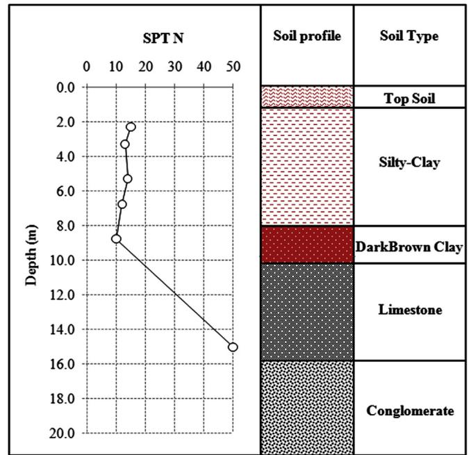
Fig. 2. Average SPT(N) values measured from borehole drillings.
