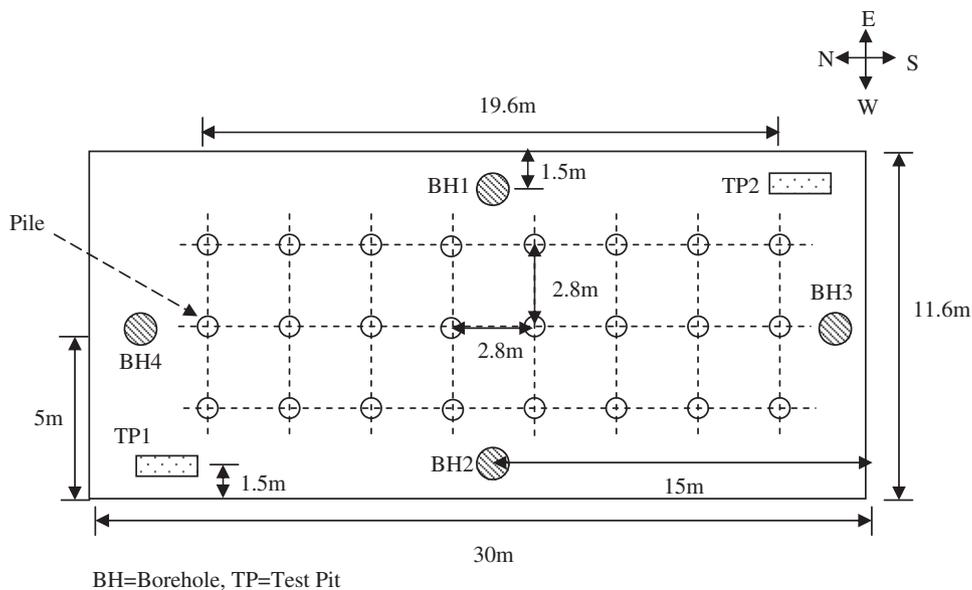
Fig. 1. Plan view showing piles, borings and test pits.
