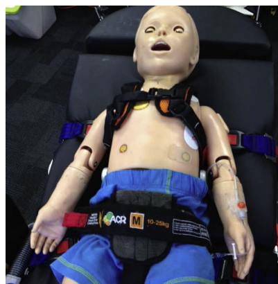
Figure 2 The five-point Ambulance Child Restraint harness used to hold a patient securely to the trolley.
