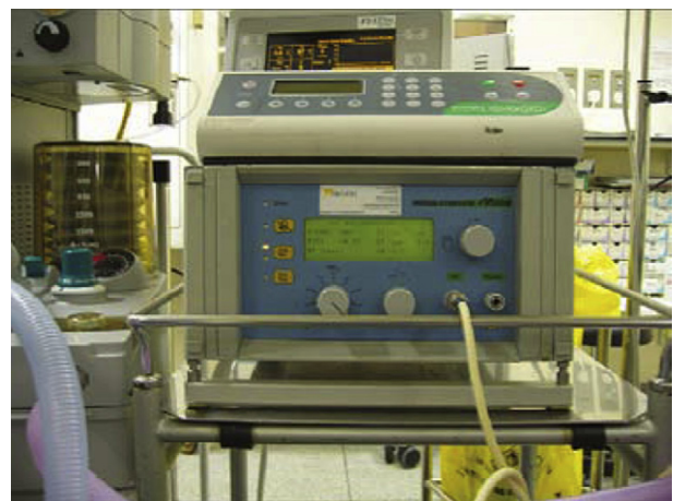
Figure 3 Mistral jet ventilator.
