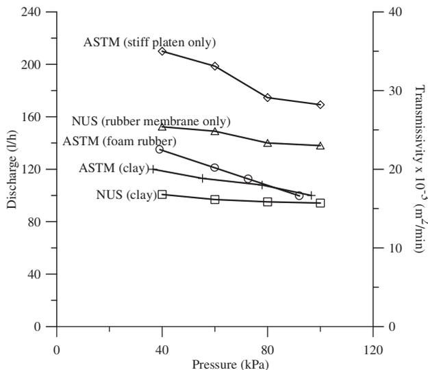
Fig. 1. PVD discharge capacity in different testing set-ups.
