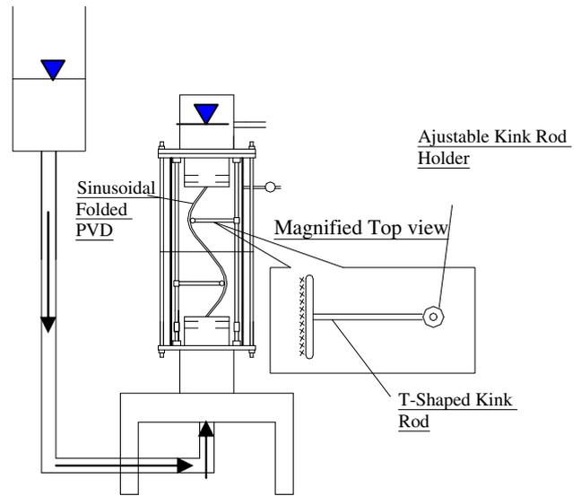
Fig. 2. PVD discharge capacity testing apparatus (NUS Ver. III) with provision for clay packing, lateral pressure, vertical and lateral deformation, and vertical water flow under constant head condition.
