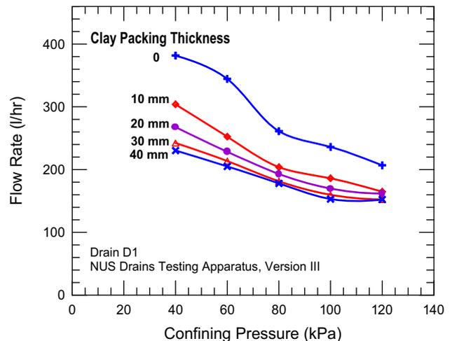
Fig. 3. Effects of lateral pressure and thickness of clay packing on drainage flow rate.
