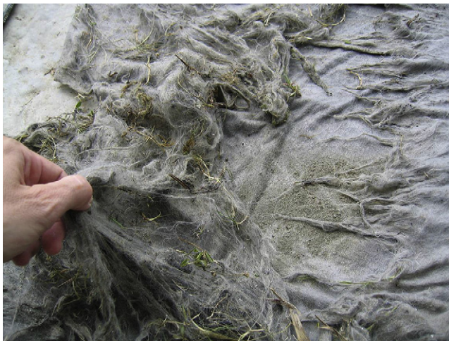
Fig. 1. A geotextile bag from the wave zone at the Bahadurabad test site on the Jamuna River. The bond between the fibers is destroyed and the bag is open. The bag was placed in early 1997, and the photo was taken in early 2005.
