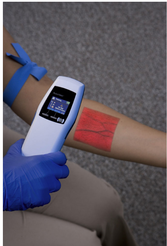
Figure 2 AccuVein AV300. An infrared device to aid vein visualization. Here the image is projected back onto the skin showing the veins as dark lines on a red background.
