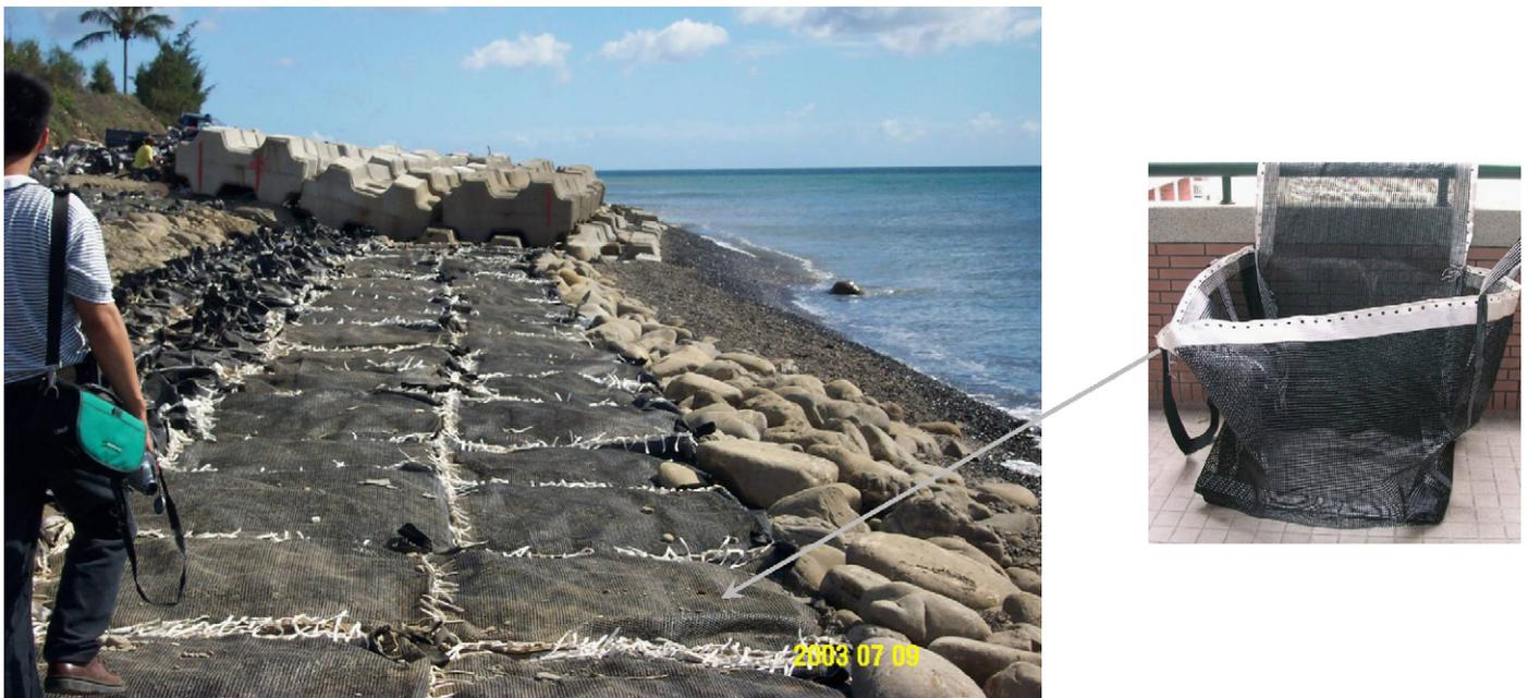
Fig. 1. Geogrid containers used in a pilot test on seashore protection.
