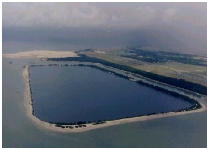
Fig. 1. Slurry pond that contains ultra-soft soil.
