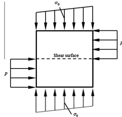
Fig. 2. Shear test specimen.
