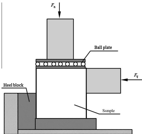
Fig. 1. Schematic diagram of shear test of rock.
