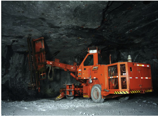
Fig. 1. J. H. Fletcher roof bolter.
