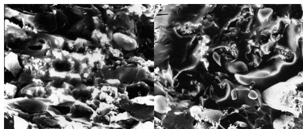
Fig. 6. Pore structure of metabituminous before and after oxidation.
