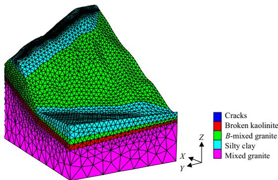
Fig. 2. Overall model of No. III landslide.
