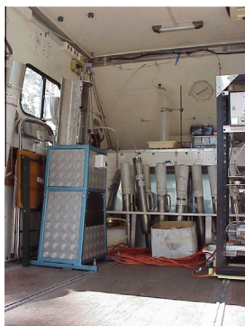
Fig. 2. CSIRO mobile gas laboratory for measurement of gas content of coal on mine site.
