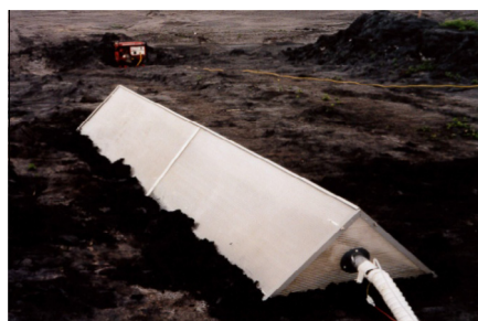
Fig. 3. Gas emitted from exposed coal into an instrumented chamber that monitors gas concentration over an extended period of time.
