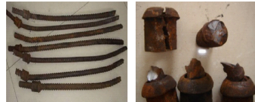
(b) Deformation and failure of shoulder bolts.
