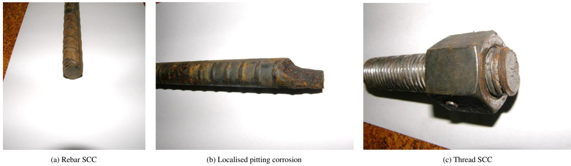
Fig. 1. Three types of rockbolt corrosion fracture surfaces.
