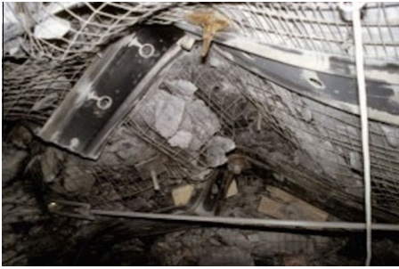
Fig. 1. A mine entry subjected to high horizontal stresses, supported with PC-strand cables subjected to combinations of tensile and shear loading.
