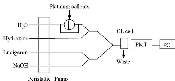
Fig. 1. Schematic diagram of flow-injection CL detection system.
