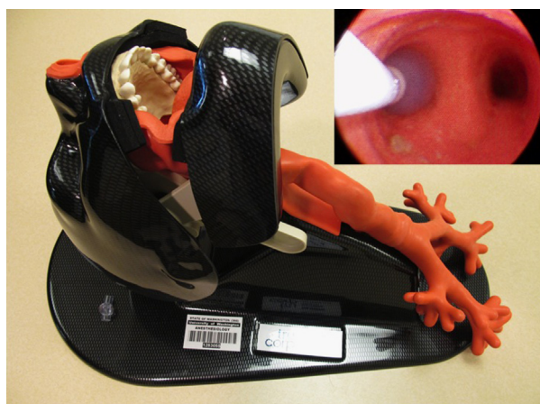
Fig 1. The AirSim Bronchi. The inset shows the view of the carina through the fiberoptic bronchoscope with a Univent blocker in the left main bronchus.
