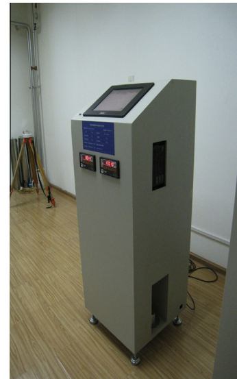
Fig. 2. Intelligent testing system for water absorption in deep soft rock.
