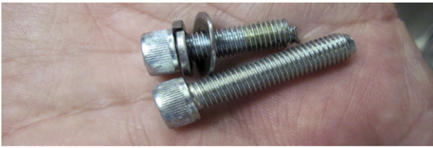
Fig. 1 One of the broken bolts (top) of the tilt cylinder mechanism compared to an intact bolt (bottom).
