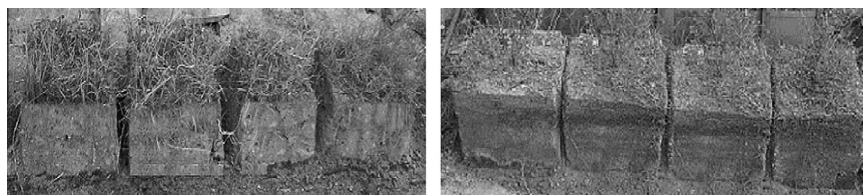
Fig. 2. Preparation of samples for shear strength test for grasses and shrubs.
