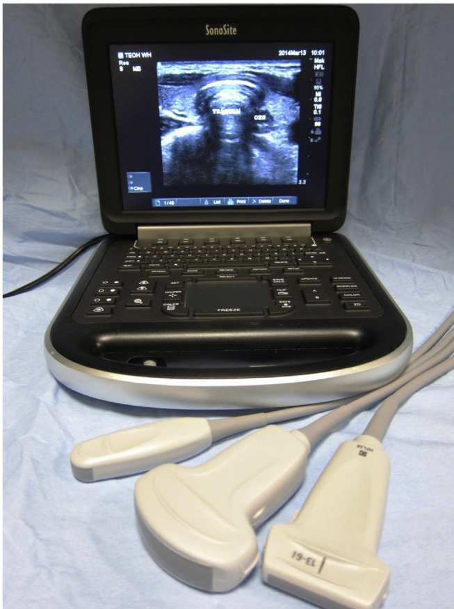
Fig. 1. A portable laptop sized ultrasound machine with transducers useful in airway management. Left to right: A microconvex transducer (5–8 MHz), a curved convex low frequency (2–5 MHz) transducer, and a linear high-frequency (6–13 MHz) transducer.
