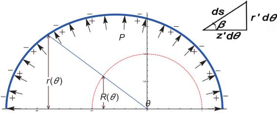
Fig. 1. Undeformed and deformed configurations of a dielectric elastomer balloon under both pressurized inflation and electric actuation.
