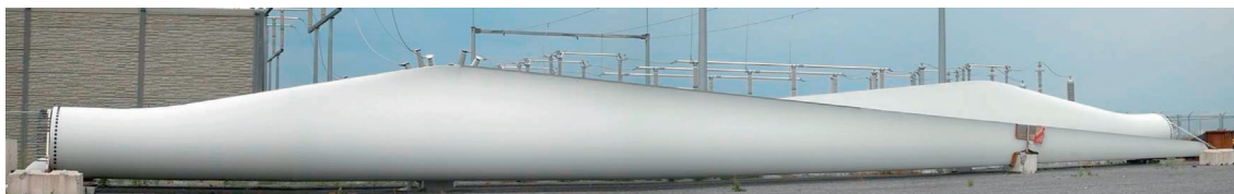
(b) Fiberglass-reinforced epoxy blades of Siemens SWT-2.3-101 wind turbines. Image from it.wikipedia.org.
