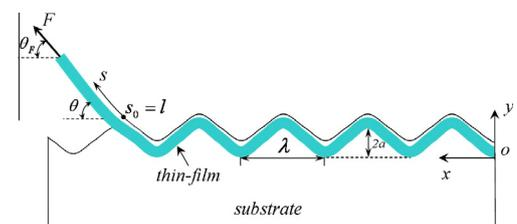
**Fig. 1.** Schematic of an elastic thin-film peeled from a sinusoidal rough substrate. The segment  $(0, l)$  of the film adheres perfectly on the rough substrate, and the part  $(l, L)$  is peeled-off under a peeling force  $F$  at a peeling angle  $\theta_F$ .  $\theta$  is the tangential angle of each point on the film with respect to a flat referred surface,  $\lambda$  is the wavelength and  $a$  is the amplitude of the roughness.
